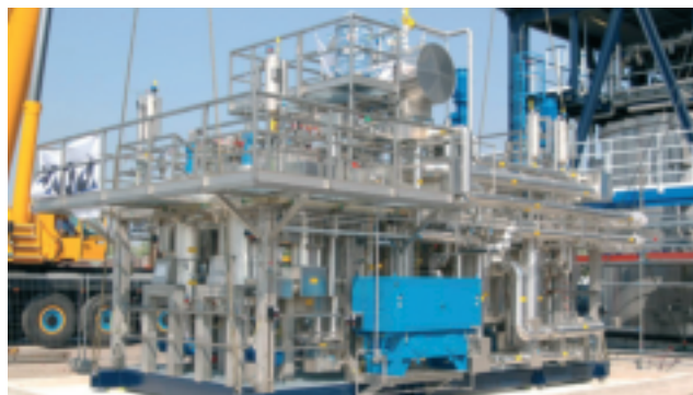
Skid mounted unit for MDI at Huntsman in the Netherlands
