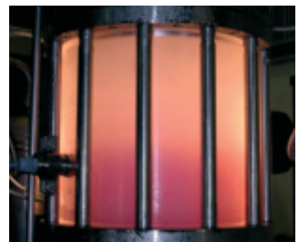
The wash column with visible wash front
